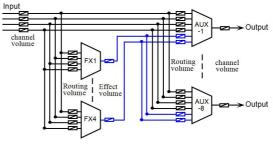
output channel resources. Each FX effects engine can independently select different effect types, which is very flexible and completely free of conflicts.
